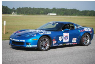
Mongoose GTP's: C4 chassis and suspension, LS7 engine, replica of 1980's Corvette GT Prototype
